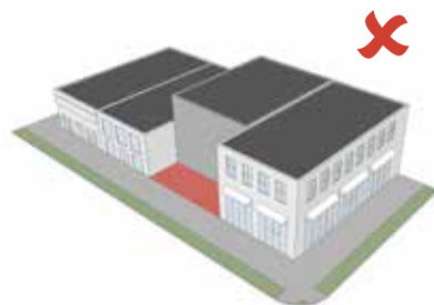
Inappropriate setback and orientation
